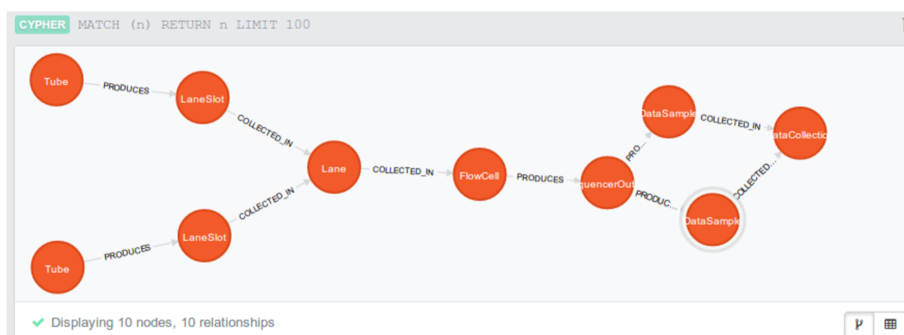
Figure 3. Diagram illustrating relationships between the sequencing objects within Omero.biobank, from the tube of DNA to the dataset ready for the downstream analyses.
